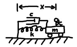
Consider a dampened mass-spring system. The Hooke's law spring force is -kx, and for our purposes damping will be proportional to velocity, so -cv. Then we have p' = (mv)' = ma = -kx - cv and  $x' = \frac{1}{m}p$ , which gives the system
